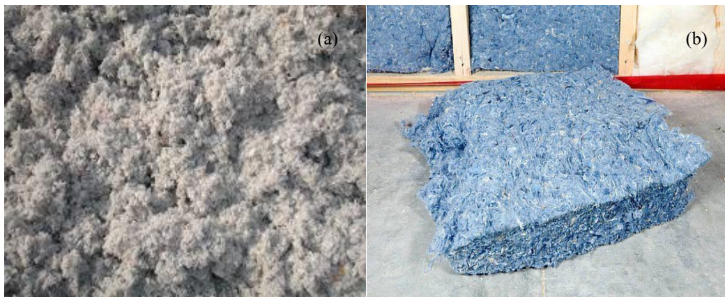
Figure II.10. Recycled insulators: (a): cellulose wadding, (b): recycled textile Source : (Guillois Isolation, 2024; Isolation-Thermique.org, 2024)
