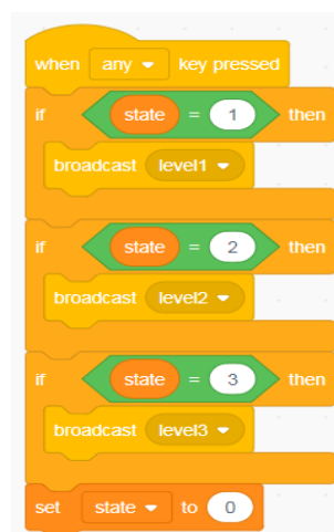
Figure 3: Active level control
