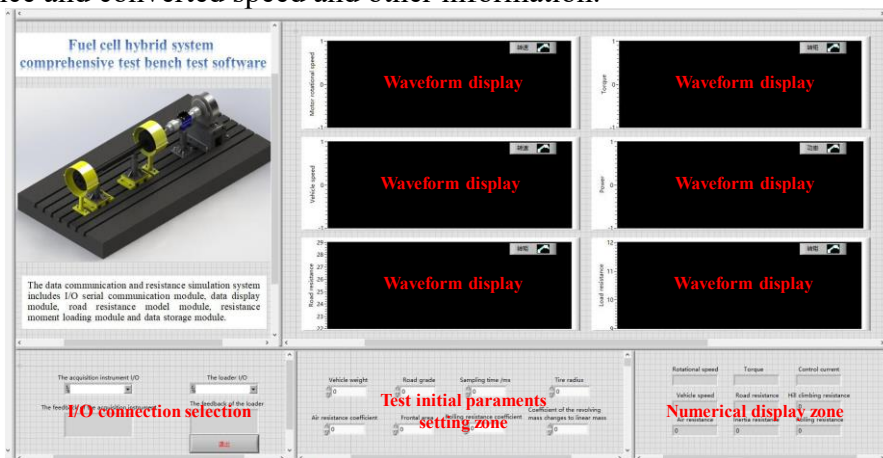
Fig. 8. Data communication and control system test interface
