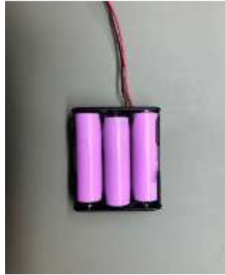
Fig. 6. Enclosure for connecting batteries in series to power the servomotors
