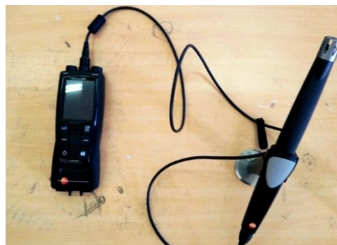
Figure 2. The used measuring instrument Testo 480 .
