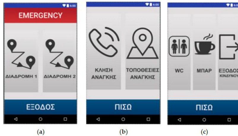
Figure 3: Blind MuseumTourer Android application activities: (a) Main menu and Route selection (b) Emergency; (c) Get voice way-finding instructions to move to the WC/canteen/exit.
