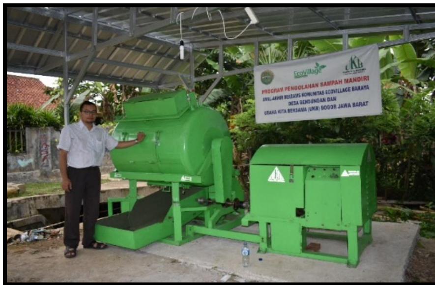
Figure 2. Briquettes and Plastic Blocks Maker as Zero Waste Program in Bendungan Village
