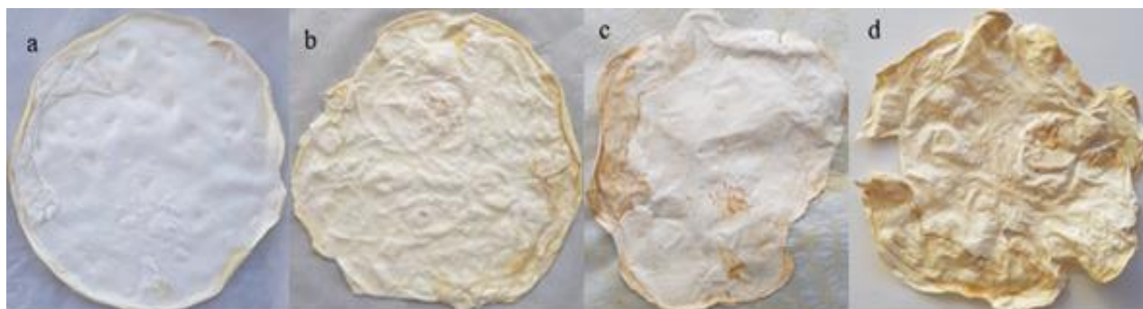
Fig. 3 Fungi leather substitute production process: (a) fresh PMM; (b) PMM after cross-link treatment; (c) PMM dried and pressed; (d) final product
