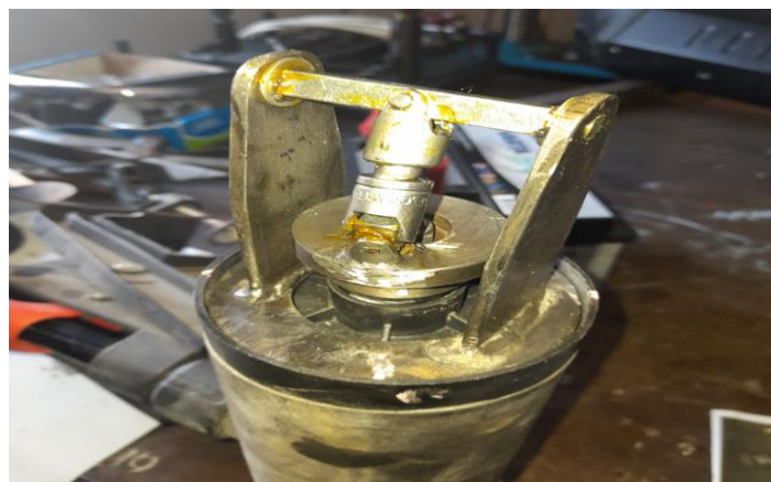
Fig. 3. The mechanical realization of the conversion of circular motion to oscillatory motion
