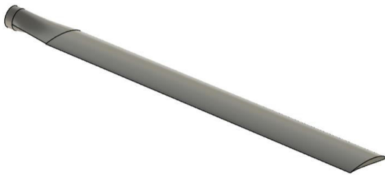
Figure 1. Modeling Blade with Airfoil SG6043 Geometry Taperless HAWT in Q-Blade Software
