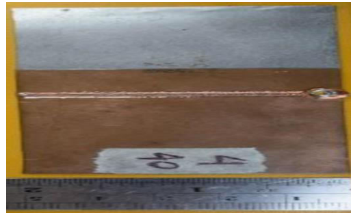
Figure 2. The best welding results with a shoulder diameter of 4mm with a welding pressure of 40kgf
