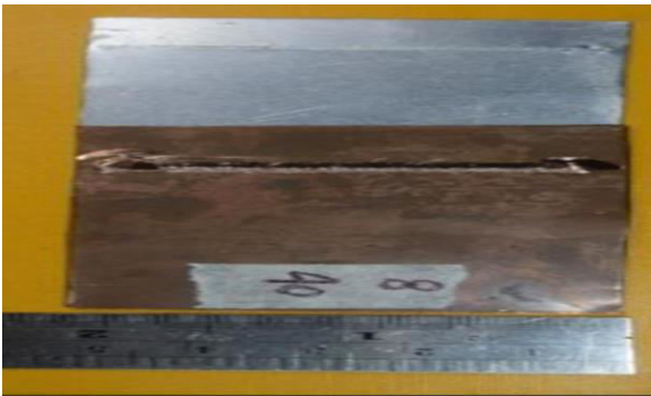
Figure 12. Results of welding with a shoulder diameter of 8mm and a welding pressure of 40mm
