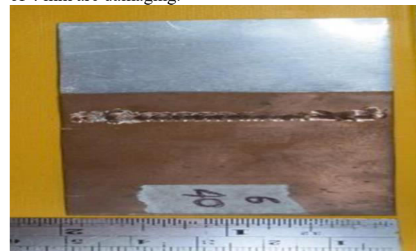
Figure 10. Results of welding with a shoulder diameter of 6mm and a welding pressure of 40kgf
