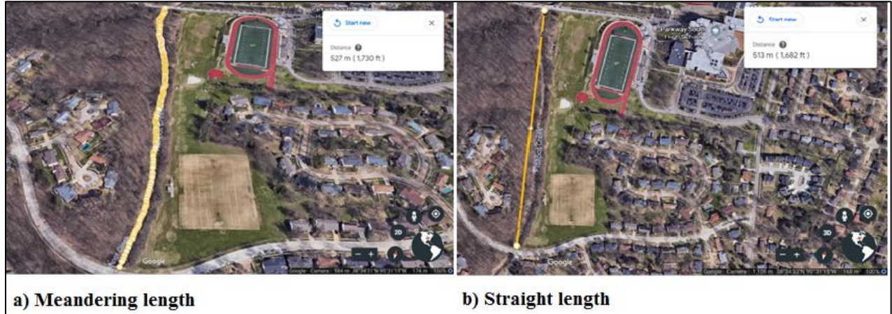
Fig. 10. Image of Google Earth showing (a) meandering length and (b) straight length estimation of Fishpot Creek
