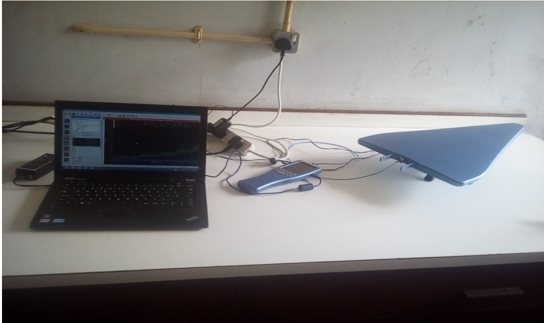
Figure 1: Experimental setup for measurement of Radiofrequency intensity exposure levels
