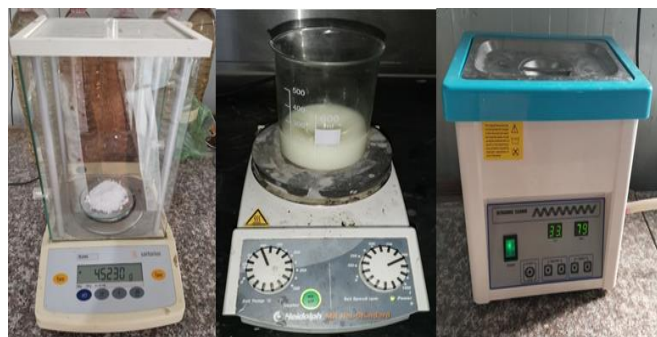
Figure2. Equipment used in the preparation of nano-fluid (a) electronic balance (b) stirring hotplate (c) ultrasonic cleaning.
