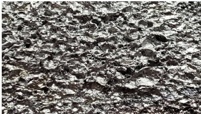
Fig.1 The general view of the sputtered coating at 4x magnification
