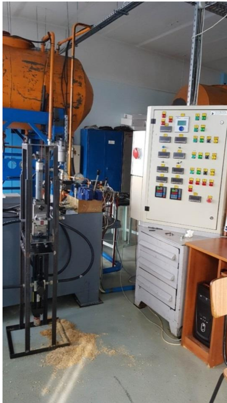
Figure 5. Active heave compensator. The experimental stand.
