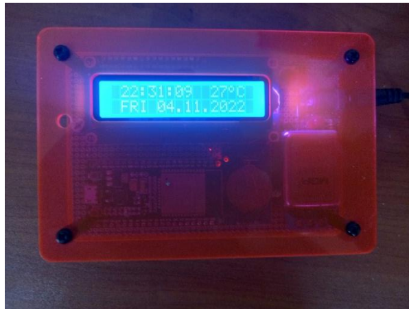
Figure 20. Displaying the actual time of the RTC on Liquid Crystal Display (LCD)
