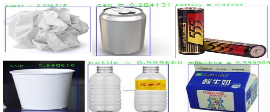
Figure 2. The average rate of recognition accuracy running on raspberry PI 3B+.
