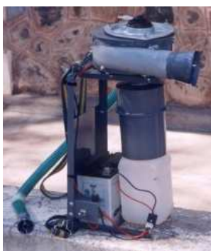
Fig. 2. Battery powered petal collector [13]
