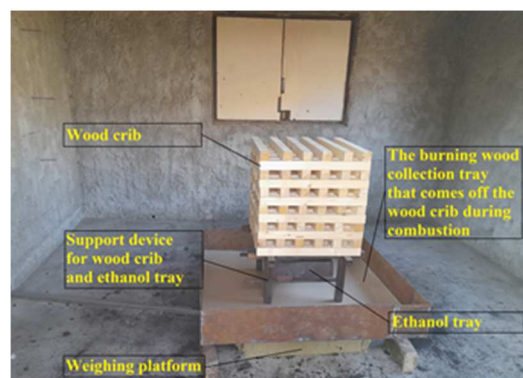
Fig. 3. Presentation of the experimental stand [16].
