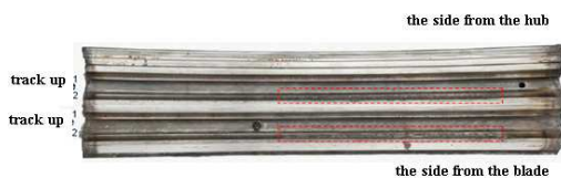
Fig. 13. Outer ring segment (top and bottom halves of raceways 1 and 2, in red - areas with major defects)
