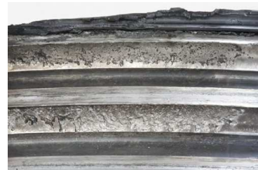
Fig. 18. Inner ring-exfoliation in the halves of the raceways
