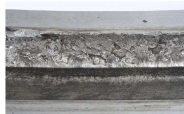
Fig. 17. Outer ring-tread with severe exfoliation
