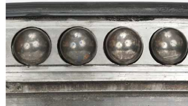
Fig. 16. Balls and cage (the cage has severe abrasion and detachment of material on the circumference)
