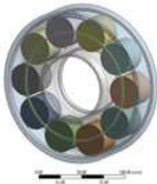
Fig. 4. The shape of the row axial straight roller bearing
