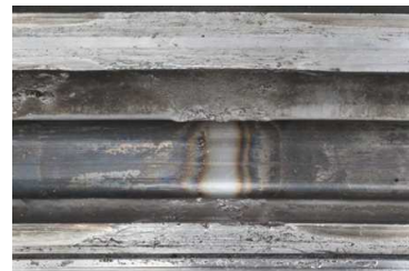
Fig. 19. Inner ring- weak points on the lower raceway
